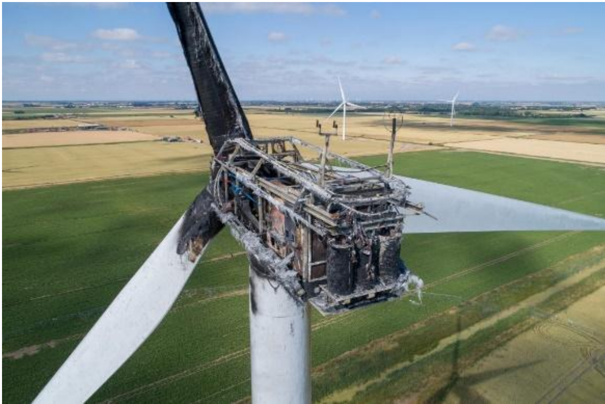
Figure 5.3.9. Damage to a WPP caused by fire. 80
